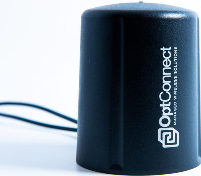
Industrial grade, versatile small size, high performing ultra-wideband cellular antenna with both a primary and diversity leads (MIMO) in a single base. Rated for outdoor use. Easy to install with a magnetic mount that can be used on any ferromagnetic (iron or steel) metal surfaces.
