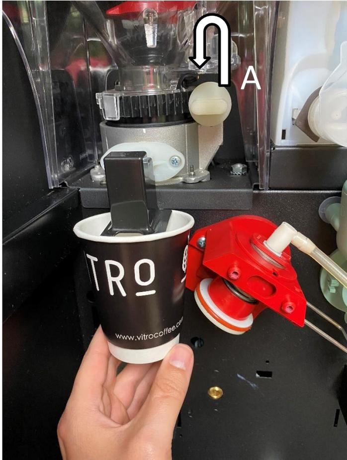
Hold a cup at the outlet of the coffee funnel use the D key to activate the grinder, let it operate for between 3-5 seconds, stop with the C key, check grind consistency.
