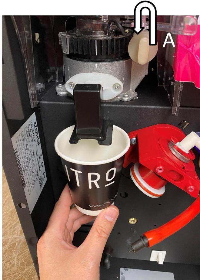
Hold a cup at the outlet of the coffee funnel use the D key to activate the grinder, let it operate for between 3-5 seconds, stop with the C key, check grind consistency.
