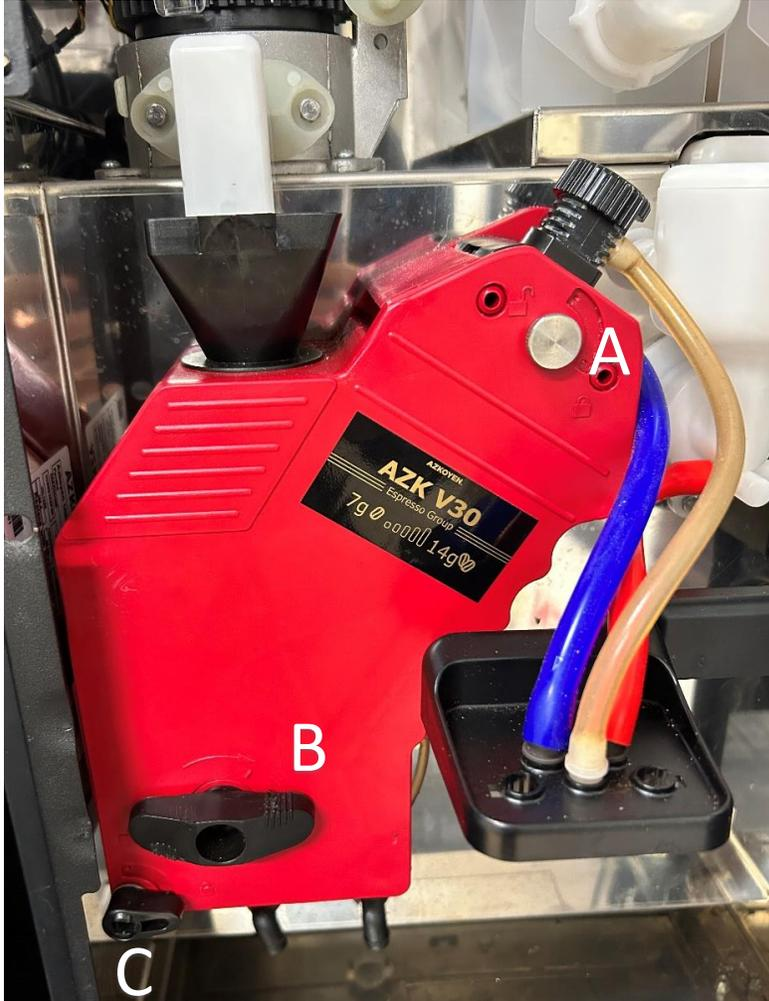
Ensure the large BLACK central handle (B) is horizontal when re-attaching the brewer body to the machine.
