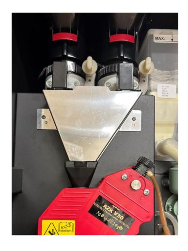
Re-attach the coffee chute to the machine using the two screws initially removed
