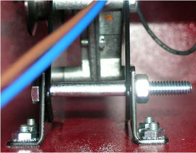
9. Remove the motor from the bracket.
