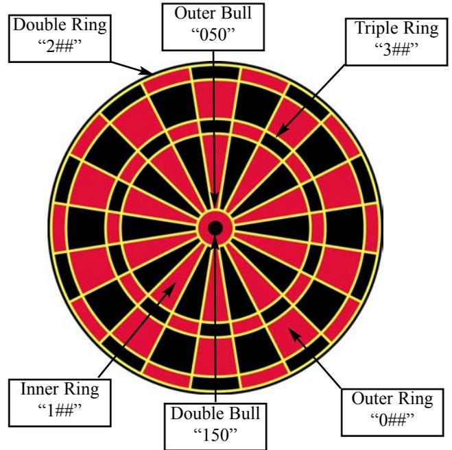
2. Tap any segment. A three digit number will appear on the display. The first number tells you which ring the segment is in. The second set of numbers tells you which pie the segment is in. Example: If **120** appears on the display, it means that the inner 20 was hit. If **315** appears on the display, it means that the triple 15 was hit.
