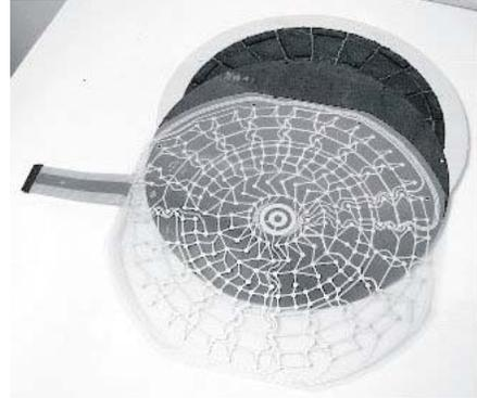
12. Check for dirt, broken tips, or other foreign matter between the spider, segments, matrix cushion, and switch matrix. Check and remove any broken tips inside the segments. Remove the segment back cover by gently prying it up. Empty the contents. Snap the cover back in place when finished.
