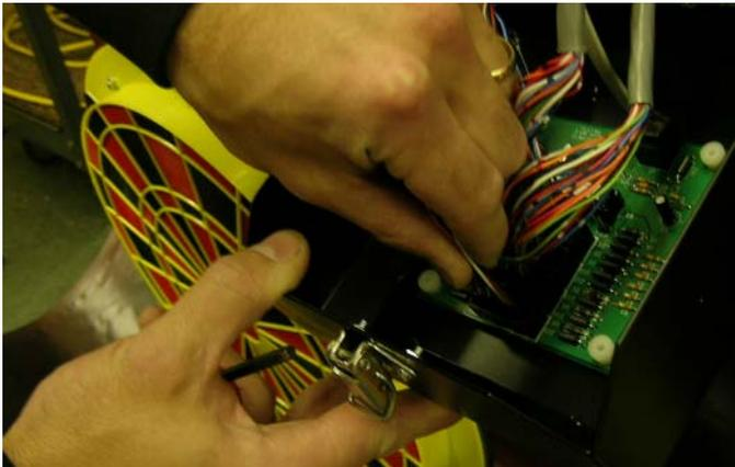
4. Loosen the socket head bolts on the darthead arm bracket.
