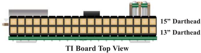
When connecting up the Switch Matrix Membranes to the TI Board, make sure the 13" darthead is plugged in to the bottom pins on the J2 connector and the 15" darthead is plugged into the top pins of the J2 connector.
