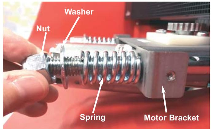
6. Using a  $\frac{3}{4}$ " wrench, tighten the hex nut to compress the spring. The compressed spring should measure  $1\frac{5}{16}$ " from the bracket to the spring side of the washer. Compress both springs evenly. This keeps the tension on the motor even, throughout the installation process.
