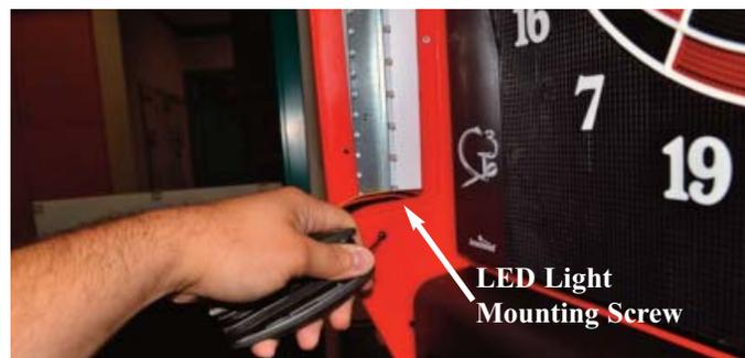
6. Pull out LED light bracket through the opening.
