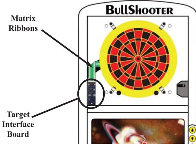
Note: You can only do this test from the 15" side. There is no way to easily access the Target Interface Board from the 13" side. This instructional will show you how to test both sides from the 15" side.
