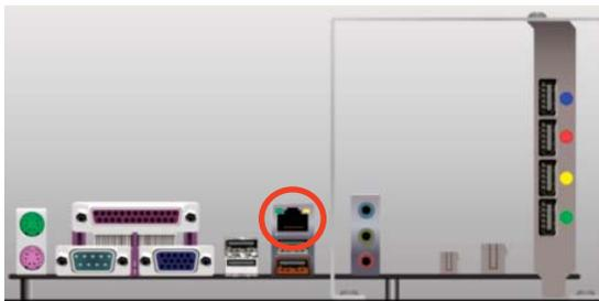
1. Run an Ethernet cable from the router to the machine.
