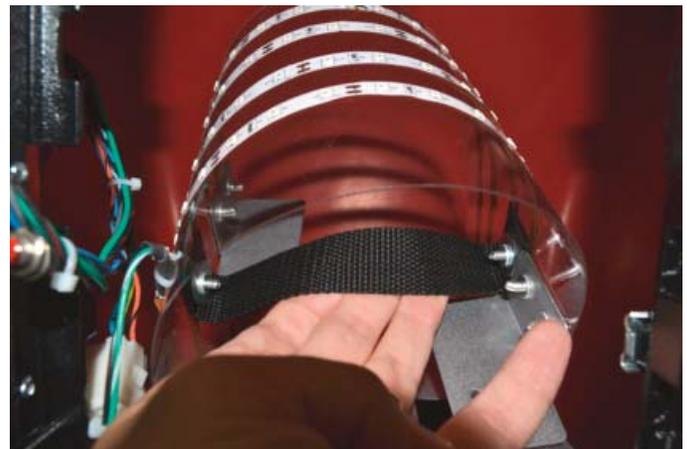
*Caution: The LED's on the hoop can get snagged on the coin door so make sure to squeeze the hoop in a little bit to get it out the door carefully.*
