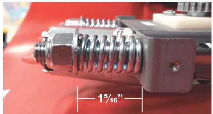
**Warning:** Be sure to tighten the springs to the exact length. If they are uneven, too loose or too tight, you could damage the motor.
