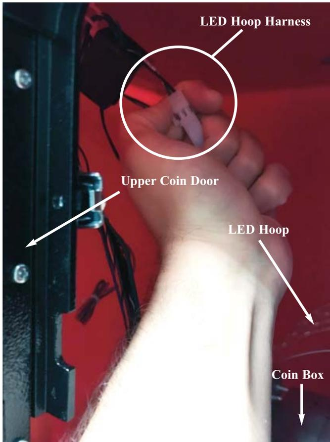
5. Cut off the wire tie from the harness. Careful not to cut other wires.
