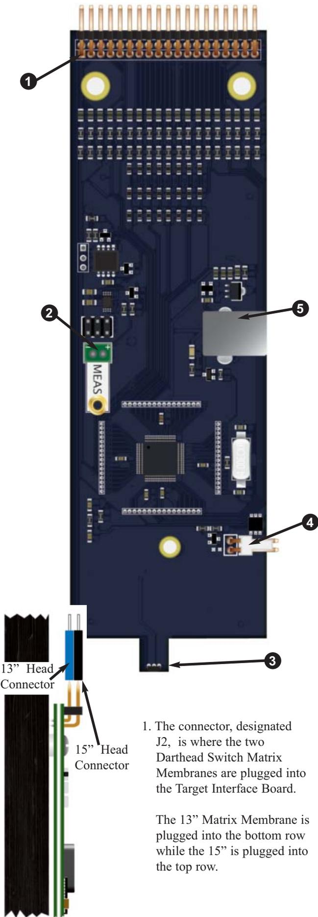
1. The connector, designated J2, is where the two Darthead Switch Matrix Membranes are plugged into the Target Interface Board.
